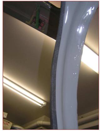
These photos show hope I filled the gaps between the door and the canopy. In the first, you can see the packing tape wrapped around the door perimeter. You can also see where I forced an epoxy / flox mixture between the canopy and door. This effectively sealed the gap. I did this a section at a time over a couple of days so as not to make the door too difficult to open. Although the epoxy doesn't adhere to
