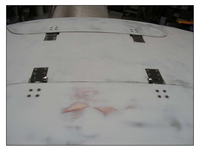
The cabin top hinge pockets where also filled in to fit snugly around the hinges. This was achieved by applying packing tape over the hinges, bolting them in place and filling the void with epoxy and flox. If you opt for this modification, make sure there is enough area around the hinge for the thickness of the paint; otherwise you'll be left with a paint ridge after the aircraft has been painted.
