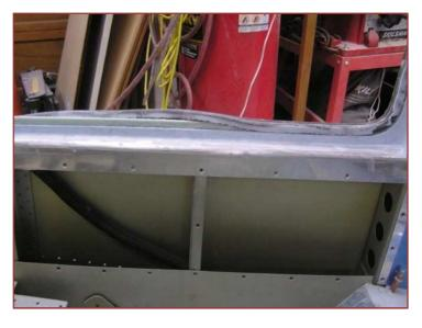
The second photo shows the result after sanding (following removal of the seal).
