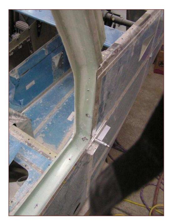
I should have mentioned that on the previous photo, it shows how all of the outward facing radii around the door opening have been cut away, this allows the seals material to sit square within the door opening, with the compression bulb facing outward towards the door.
