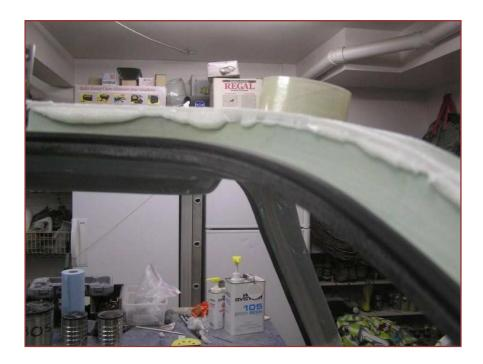
This shows how I got the door and canopy on the same "plane". I closed the door and then speed an epoxy / micro balloon mixture across the transition from the door to the canopy. Low areas on either the door or canopy were filled.
