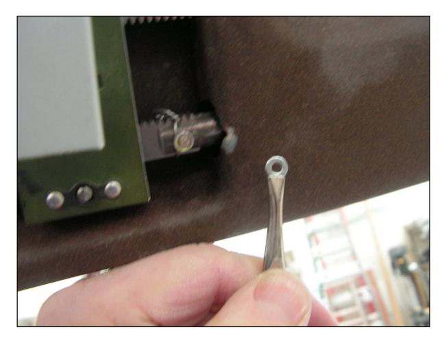
One other modification involved getting the door hinges chrome plated by a local shop and replacing the supplied steel screws with structural stainless hardware from Aircraft Spruce. The two bolts which secure the front shoulder harnesses to the cabin tap can also be chrome plated, to improve the aesthetics of the installation.
