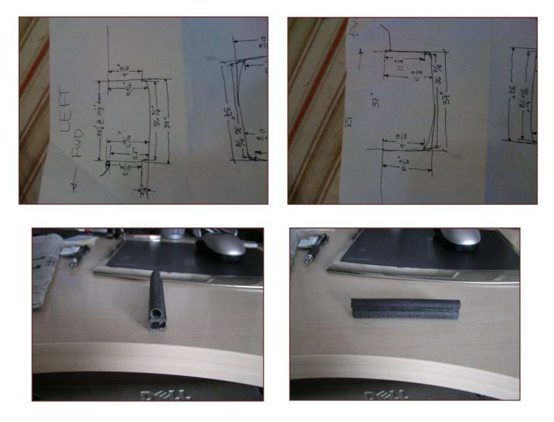
The pictures above show a short length of the McMaster Carr seals (Part #1120A313) as well as an end on shot. The edge grip is solid and fits onto the door sill opening, whilst the rubber bulb is compressible against the closed door, forming a tight weatherproof seal. You'll need about 100 feet to do the job and have some spare.
